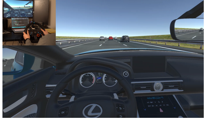
Fig. 4: Naturalistic driving in a car-following scenario with Unity game engine and Logitech racing wheel.
