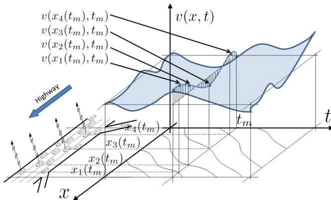
Figure 1. Illustration of the distributed velocity field  $v(x, t)$  to be reconstructed from Lagrangian samples. Four samples  $v_i(x_i(t), t)$  are shown at  $t = t_m$ , from vehicles  $i$  transmitting their data (indicated by up-arrows above the vehicles).
