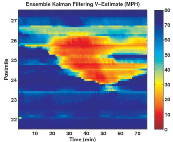
Figure 5. EnKF velocity contour plot, I880N, Feb. 8, 2008. Color denotes speed in mph, with red denoting slow moving traffic, and blue denoting faster traffic. Vehicles travel from down to up.  $x$ -axis: time in minutes past 10:12am.  $y$ -axis: postmile between Decoto Rd. to the south (bottom) and Winton Ave. to the north (top).
