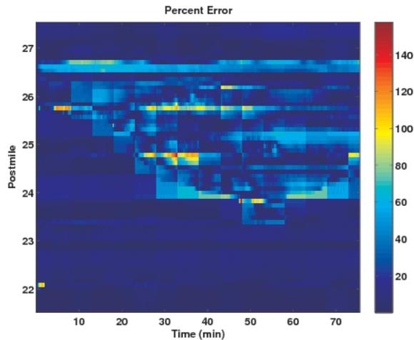
Figure 7. PeMS-EnKF error Plot, I880N, Feb. 8, 2008. Color denotes speed in mph, with red denoting slow moving traffic, and blue denoting faster traffic. Vehicles travel from down to up.  $x$ -axis: time in minutes past 10:12am.  $y$ -axis: postmile between Decoto Rd. to the south (bottom) and Winton Ave. to the north (top).
