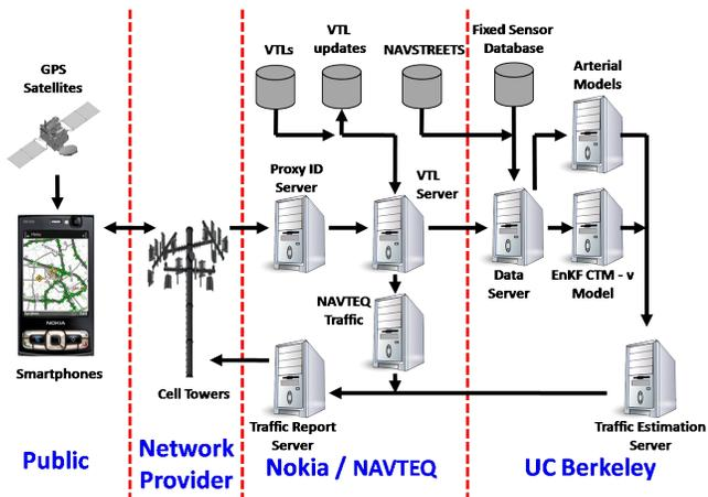
Figure 2. System architecture overview. The system consists of vehicles equipped with GPS-enabled smartphones, a cellular network provider, an ID data collection infrastructure and traffic information provision, and traffic estimation algorithm running on the model server.
