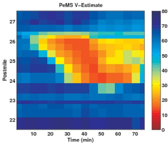
Figure 6. PeMS velocity contour plot, I880N, Feb. 8, 2008. Color denotes speed in mph, with red denoting slow moving traffic, and blue denoting faster traffic. Vehicles travel from down to up.  $x$ -axis: time in minutes past 10:12am.  $y$ -axis: postmile between Decoto Rd. to the south (bottom) and Winton Ave. to the north (top).
