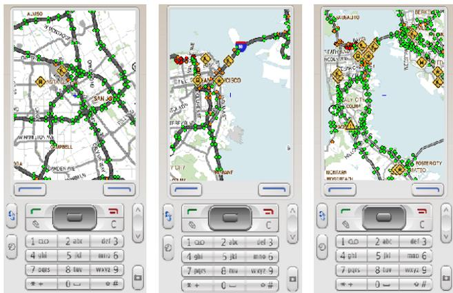
Figure 3. Nokia N95 client emulator used for development of our system. The client serves both to collect data from individual devices, and to display current traffic conditions. The colors in the circles represent the speed of traffic (green corresponds to free flow; red is congested). (Left) Free flowing traffic in Santa Clara, CA. (Middle) Congestion occurs in San Francisco, CA. (Right) Bay Area regional traffic.
