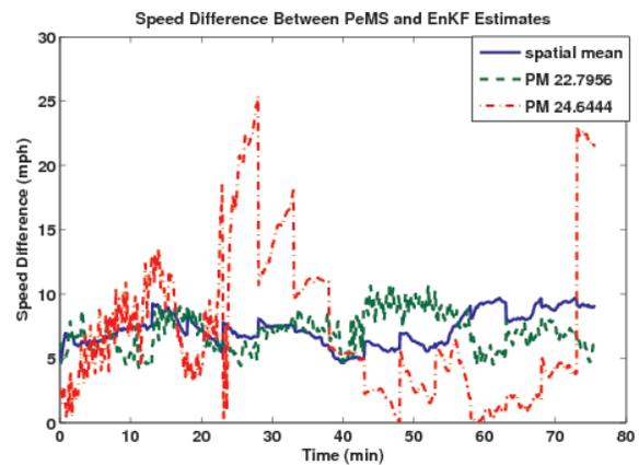
Figure 8. PeMS-EnKF speed difference, I880N, Feb. 8, 2008. Absolute difference in the velocity estimates between EnKF and PeMS spatially averaged across the network (solid blue), at postmile 22.8 with low relative error (dashed green), and postmile 24.6 with high relative error (dash dot red) as a function of time.  $x$ -axis: time in minutes past 10:12am.  $y$ -axis: absolute speed difference between EnKF and PeMS.
