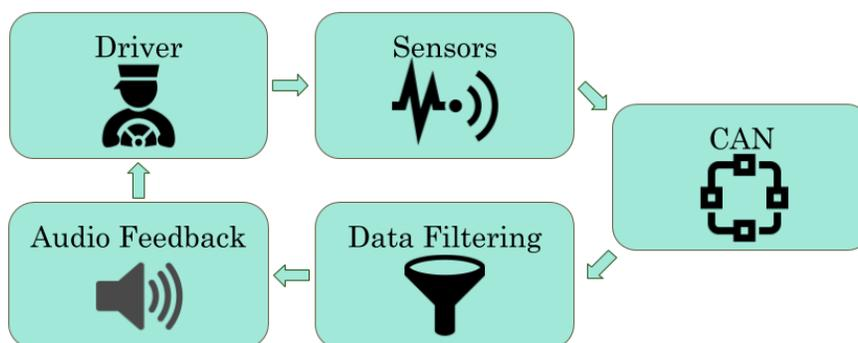
**FIGURE 1** : CAN Coach system. Stock sensors on the vehicle report measurements on the CAN, which are used to determine the error between a desired time gap (to the car ahead) control objective and the current time gap. The magnitude and direction of the error is fed back to the driver, who adjusts the vehicle. The changes are measured by the sensors and the feedback loop is closed.
