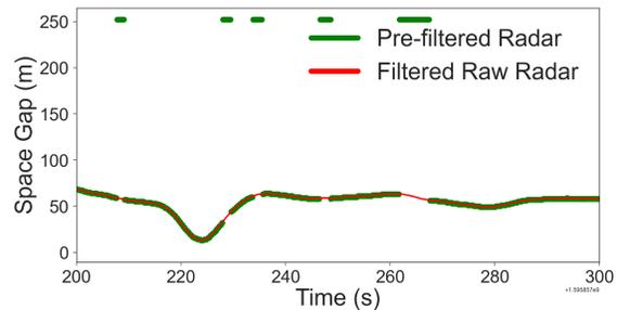
(d) Filtered raw radar sensor data overlaid with pre-processed radar.
