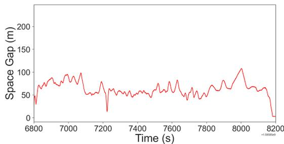
(c) Filtered raw radar space gap data.
