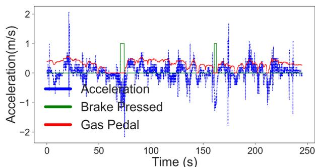
**FIGURE 3** : Acceleration, gas, and brakes signals during the Normal Driving Low Dips test. Brake Pressed is a binary signal indicating if the brake is pressed. Gas Pedal is a proportional signal from 0-1.
