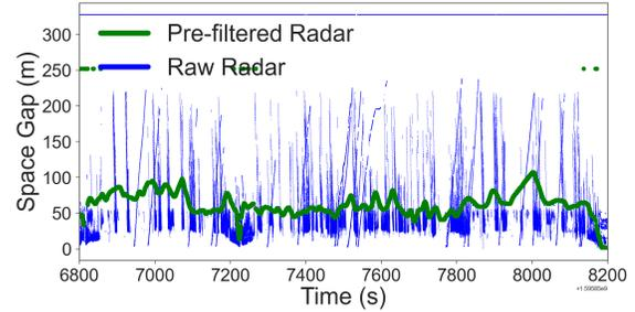
(b) All raw radar space gap data with pre-processed radar overlaid.
