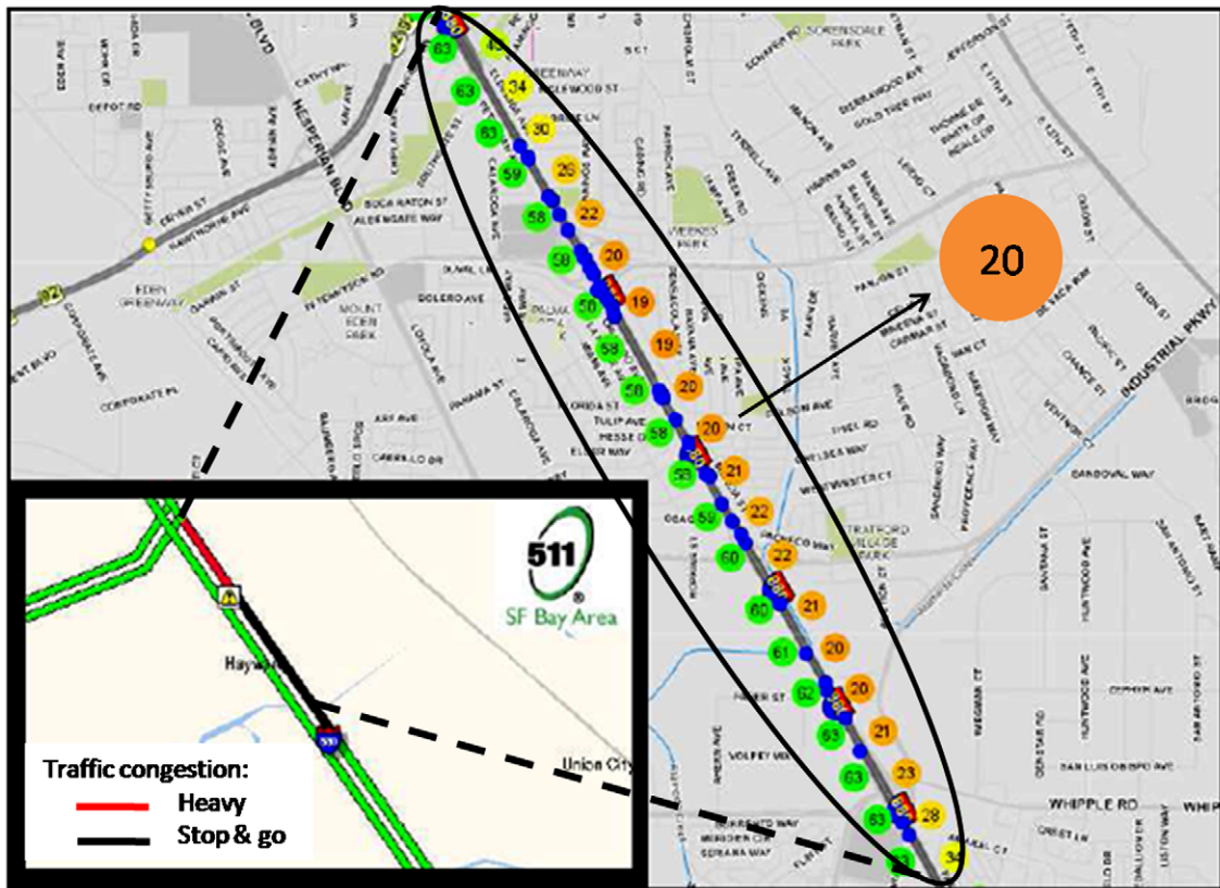
Fig. 3. Live traffic feed at 10:52 am on February 8, 2008, after an accident on the NB direction of I880 occurred, provided by the proposed system and 511.org (inside). Numbers in circles correspond to speed in mph.
