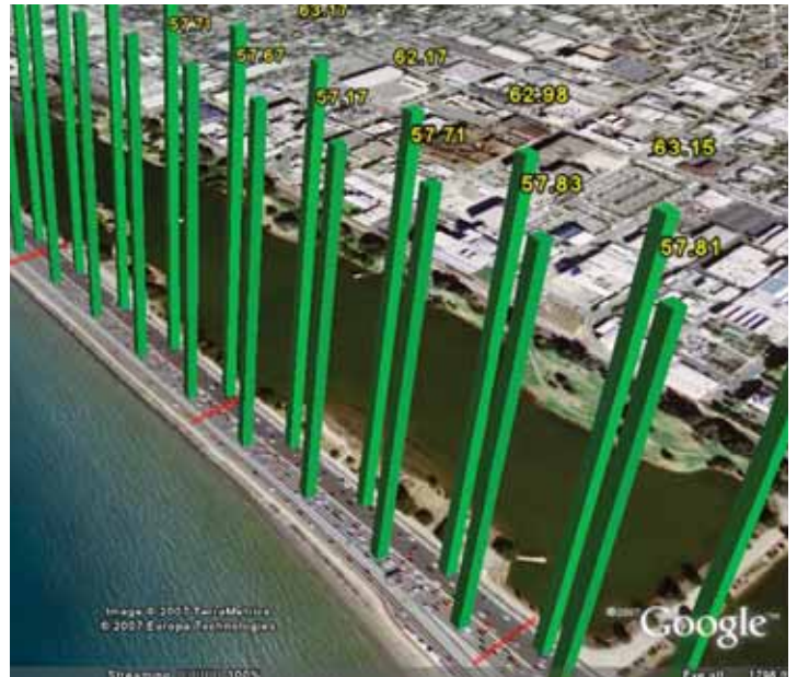
A Google Earth rendering of collected GPS data. Virtual trip lines (shown in red) trigger measurement updates to the server.
