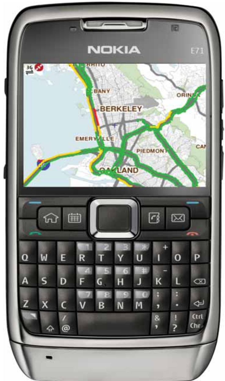
A Nokia E71 Smartphone shows Mobile Millennium Traffic Pilot software displaying real-time freeway traffic in Berkeley, CA.
